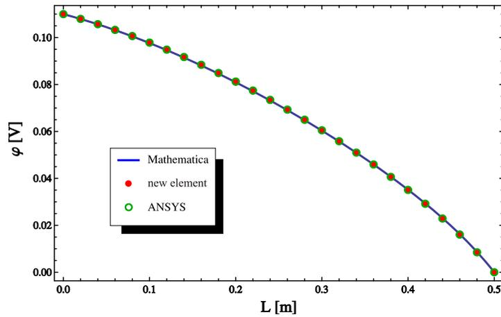
Fig.2: Distribution of the electric potential through the length of conductor.
