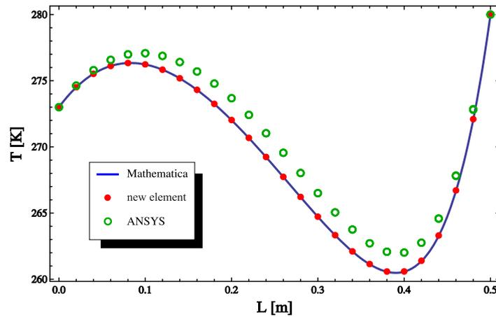
Fig.2: Distribution of the temperature through the length of conductor.
