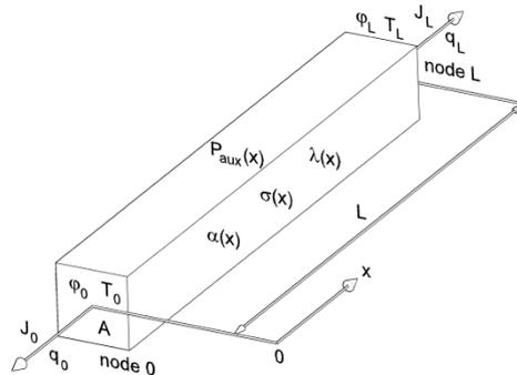
Fig.1: Two-nodal conductor for thermoelectric analysis.
